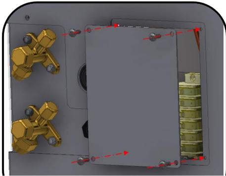
Step 1: Unscrew and remove the electrical access plate of the outdoor unit.
