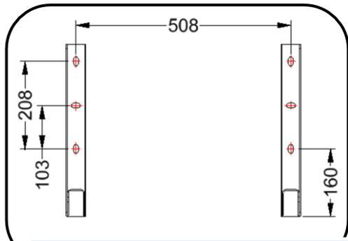
Step 1: Mark out and drill the fastening holes as indicated. (Drilling diameter: 12 mm max.)
