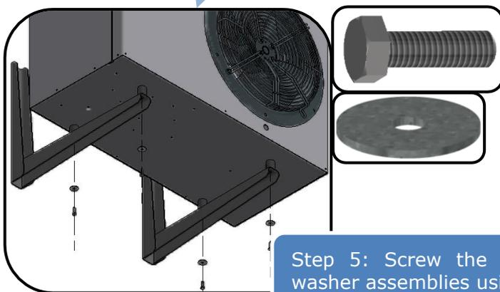
Step 5: Screw the four M6 bolt and washer assemblies using a 10 mm key.
