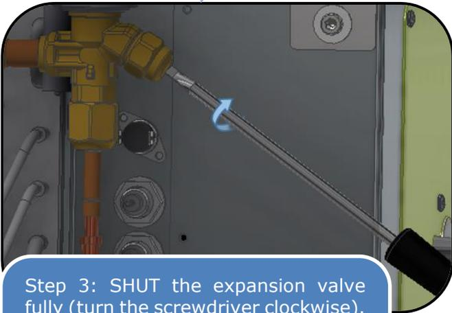
Step 3: SHUT the expansion valve fully (turn the screwdriver clockwise). Check the position of the tip of the screwdriver (to give it the right number of turns for correct expansion valve adjustment)
