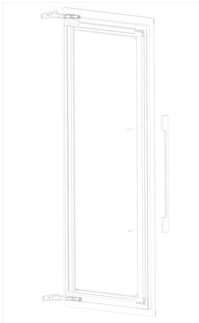
If the screws holes of the handle don't match perfectly with the holes of the door, please use an electric drill to drill the holes of the door a bit big (in surface side), in order to install the handle perfectly.
